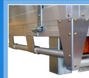
40mm Alloy Rope Rails & Alloy Corner Trim
