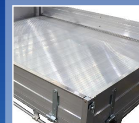
32mm Thick Alloy Flooring
