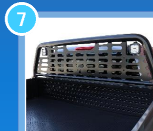
4mm Laser Cut, Fully Welded Window Guard
