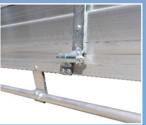
Tapered Hinge Pins + Rope Rail
