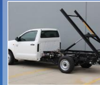
Heavy-Duty Steel Powder Coated Sub Frame
