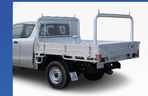
90° 76mm Alloy, Pod-Mounted. 1360mm Between Pins.
