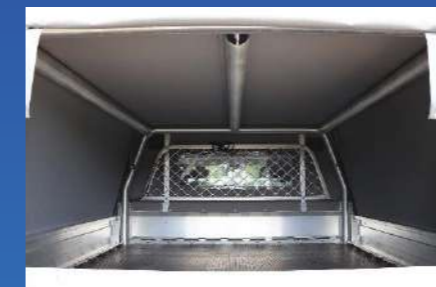
3 x 76mm Heavy-Duty Alloy Removable Stabiliser Bars
