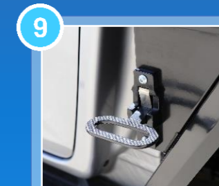
Fold Down Step on Both Sides of Tray
