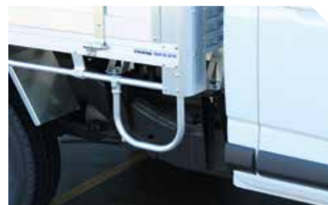
Step Kit Single- Fleet & Tradesman 25mm diameter (Not suitable for Crew Cabs)
