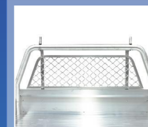
Alloy Headboard + Mesh Headboard Panel
