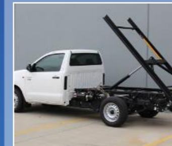
Heavy-Duty Steel Powder Coated Sub Frame
