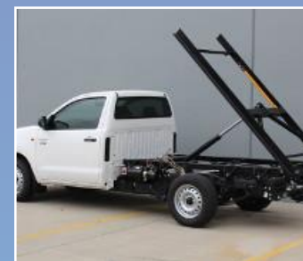
Heavy-Duty Steel Powder Coated Sub Frame
