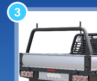
76mm Powder Coated Rear Rack to Match Headboard
