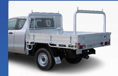
90° 76mm Alloy, Pod-Mounted. 1360mm Between Pins.
