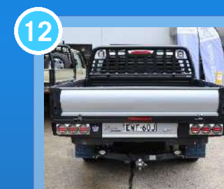
Number plate mounted in centre of Trundle Tray face
