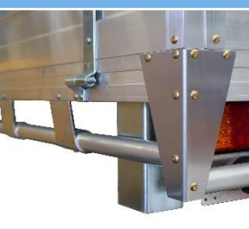
40mm Alloy Rope Rails & Alloy Corner Trim
