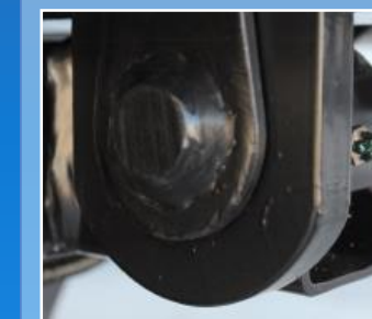
Strong 30mmØ pin with grease nipple
