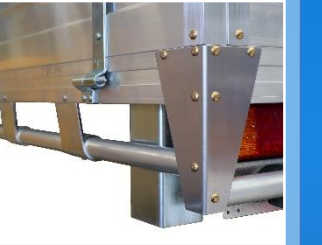
40mm Alloy Rope Rails & Alloy Corner Trim
