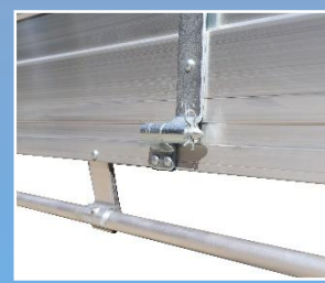
Tapered Hinge Pins + Rope Rail
