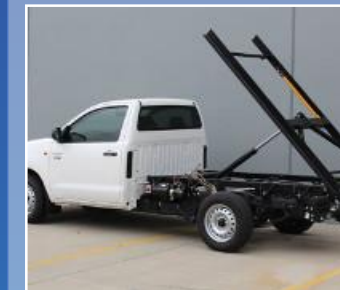
Heavy-Duty Steel Powder Coated Sub Frame
