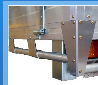
40mm Alloy Rope Rails & Alloy Corner Trim
