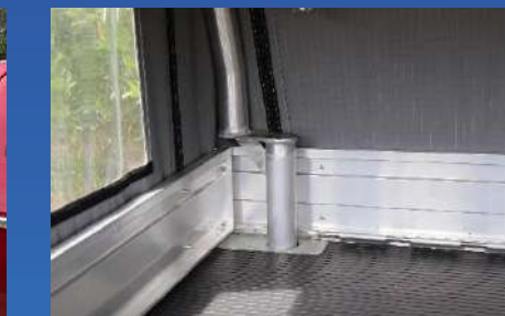
Offset Rear Rack Modification to Allow the Canvas to Fit Neatly Over the Rear of the Tray
