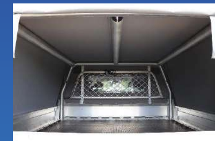
3 x 76mm Heavy-Duty Alloy Removable Stabiliser Bars
