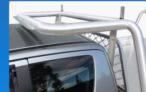
76mm Round Alloy Tube. 650mmW Wind Deflection Fin.
