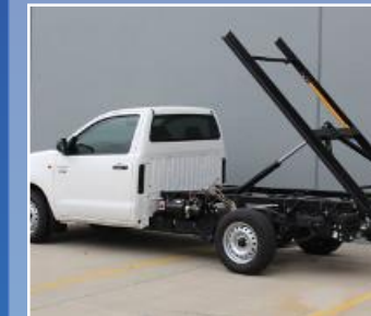
Heavy-Duty Steel Powder Coated Sub Frame
