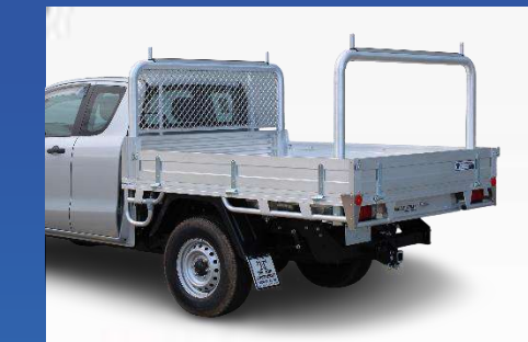
90° 76mm Alloy, Pod-Mounted. 1360mm Between Pins.
