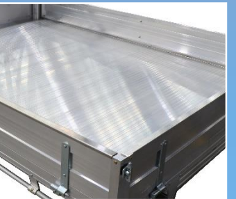
32mm Thick Alloy Flooring
